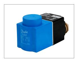
EEC electronic coil controller for solenoid valves, The EEC gives the coil a short over-boost, and controls the armature speed:
