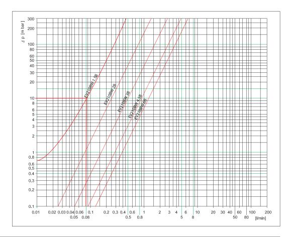
Example, water at higher pressure: Capacity for EV210BW 1.5B at differential pressure of 1.5 bar. Approx. 0.1 m³/h
