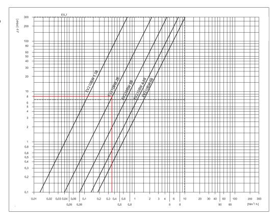
Example, air at higher pressure: Capacity for EV210BW 2B at inlet pressure (p1) of 5 bar and outlet pressure (p2) of 3.25 bar.
